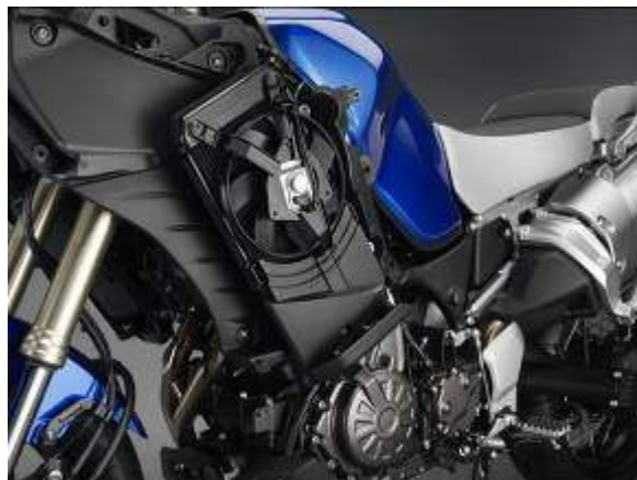
Side mount radiator allows a more compact design and aids mass centralisation for improved handling
